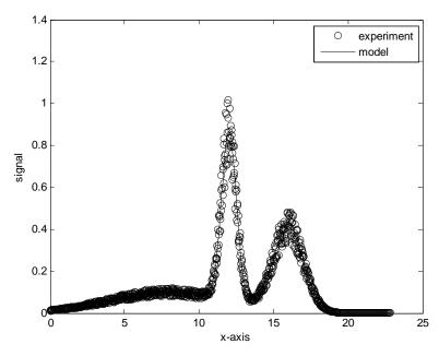
It appears to me that three curves are necessary. From this plot, I chose initial guesses of 6, 11 and 15 for the three means and 3, 3 and 2 for the standard deviations. (These are not particularly good initial guesses.)
