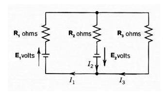
Circuit analysis is performed by using Kirchoff's Current & Voltage laws. Kirchoff's current law states that the sum of the currents entering and leaving any node must sum to zero. So for the bottom node, Kirchoff's current law provides the following equation.
