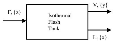
This unit takes a pressurized liquid, two-component feed stream and exposes it to a low pressure vessel maintained under isothermal conditions. The net result is that some of the fluid is vaporized, while some fluid remains liquid. The compositions of the liquid and vapor phase are determined by the combined analysis of mass balances and Raoult's Law for vapor-liquid equilibrium. The temperature in the flash tank is T = 298 K and the pressure in the tank is P = 101 k P a.
